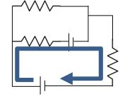
Upper loop:  $10 V - I_3 (15 \Omega) - I_1 (20 \Omega) = 0$
